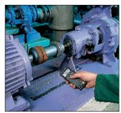
rpm measurement on shafts
