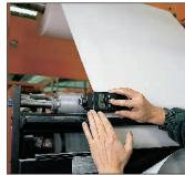
Mechanical rpm measurement on a roller
